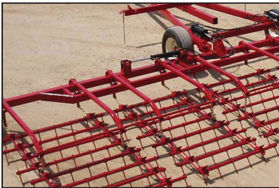
Trussed wing eliminates wing cable & wings float up/down in uneven terrain.
