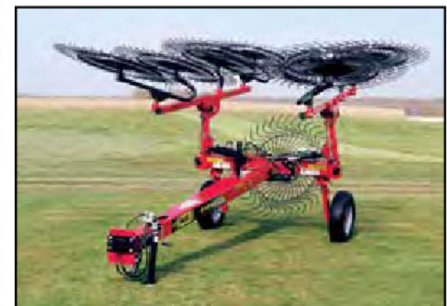
Rake in transport position with optional Center Kicker Wheel. 2200 series rake shown.
