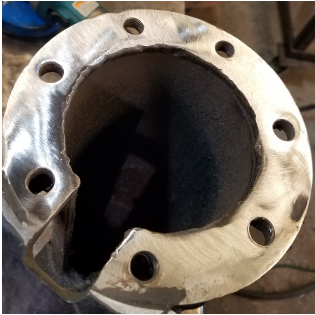
Fig. 4: Flange restored to its original surface profile
