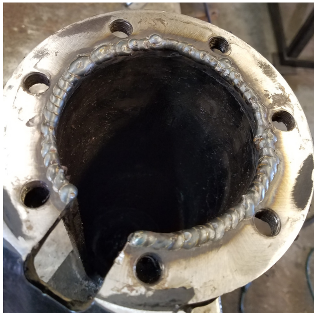
Fig. 3: Spot welds around flange circumference
