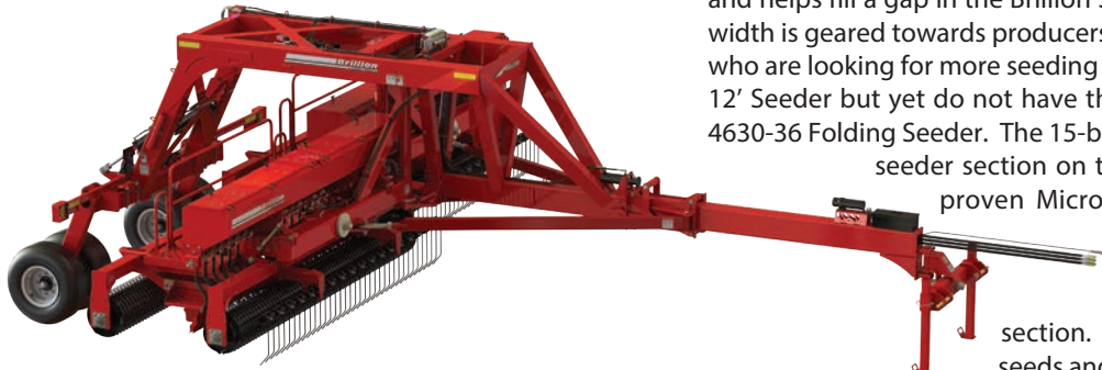
Model 4620-24 Shown with Optional Coil Tine Track Remover Kit
