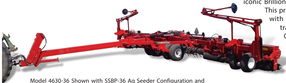
Model 4630-36 Shown with SSBP-36 Ag Seeder Configuration and Optional Folding Row Marker Kit
