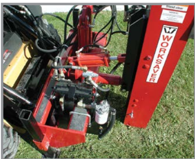
Self-Contained Unit — Overhead view of compact design (required for select models of skid steers, available for all size drivers)
