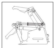
The SARG with its 66 degrees of sweep allows the operator to move rocks of varying sizes into the bucket. The sweep clamp operates like a thumb moving material into and retaining it in the bucket.
