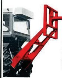
The Hi-Lift easily mounts on category II 3 point, or category III 3 point, that can be converted to category II with spacer bushings. It uses a standard 8" tractor cylinder allowing 80 degrees of movement.
