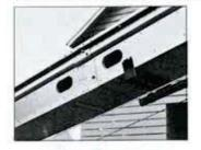
Anti-Sag Construction. Sturdy, rust-resistant galvanized steel trough sections are connected with embossed, interlocking joints. All section joints are reinforced to prevent sagging. Cadmium-plated bolts and nuts add extra corrosion resistance.
