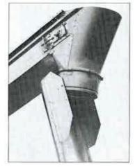
360" Swivel Head and Telescoping Spout fills crib corners. Alm the flow where you want if. Large 18" diameter opening. Telescoping 4" downspout sections increase reach up to 16". Assembly can be swung out of the way, or removed, for bale handling.
