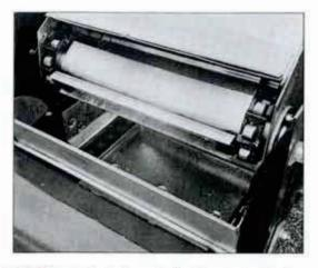
Grain Saver. A simple, yet effective device that works in conjunction with tilt-up hopper to prevent grain spillage.
