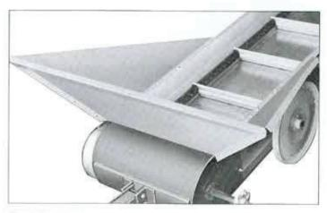
Shovel Hopper is available for use when dumping from truck or wagon. Note: Guard removed for photographic reasons.
