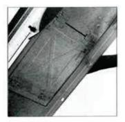
Corn Screen/Relief Door. Standard features. Located in top section of elevator for maximum cleaning. Open the relief door to allow discharge of screened material. Leave closed while elevating small grains.
