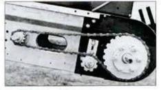
Adjustable Speed Reduction with optional Opposite Side Drive lets you drive the elevator from either side. Sip clutch can be adjusted for elevating various materials. Note: Guard
