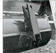
Double Clevis Hitch. Strong and rigid for towing. Change pin and swing out of the way when working.
