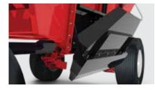
The optional center dump directs the unloading material beneath the gravity box, ideal for when the unloading area isn't wide enough for standard side dumping.
