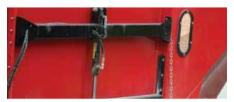
The Hydraulic Door allows you to conveniently control the metering of the material using a remote from your tractor.
