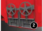
The optional divider splits your Gravity Box ①, allowing for two separate commodities to be in the box at the same time. Each side also has it's own door for individual unloading and metering ②.
