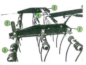
HEAVY DUTY ARM MOUNTING BRACKET INSURES STURDY MOUNTING TO CULTIVATOR OR CHISEL PLOW.
