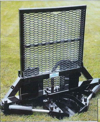
The original Tree Terminator tree shear will cut up to 14- inch diameter trees. It is designed to withstand continued use to give years of trouble-free operation.
