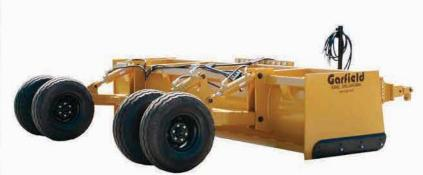
The two lift cylinders are 4" bore, 2" shaft and 12" stroke. The tires are 11L X 15. Third cylinder is for tilt models
