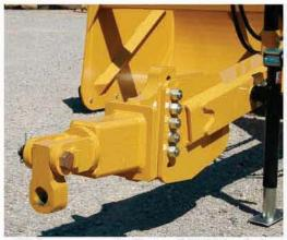
Sides are reinforced 5/8" plates. All models have 22" Ground Clearance.
