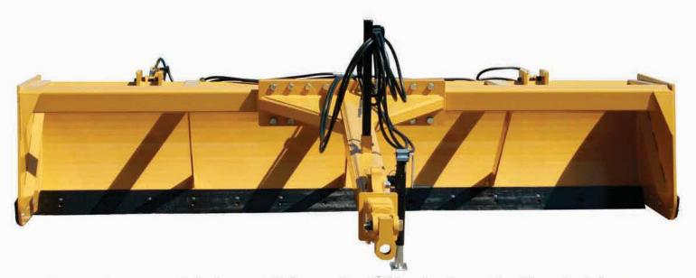
Heavy Duty models have 3/8" step broke back plate 3' tall and 4' deep. Blades are  $3/4 \ge 8$  reversible.
