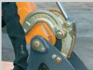
Drop forged lever for flail head rotation
