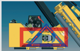
Frame "DELTA BOX" (forces shared and balanced)
