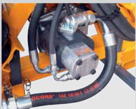
Group 3 cast iron hydraulic rotor pump
