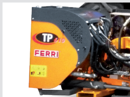
Pressurized oil tank (protection cover available on EP-Tronic controls version ONLY)
