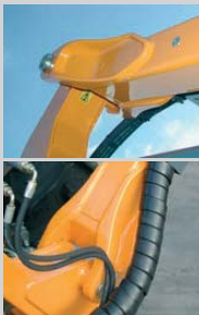
Drop forged brackets for the arms
