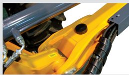
Frame "DELTA BOX" (forces shared and balanced)
