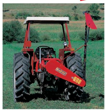
The SITREX Sickle bar Mower Series SB is a simple and reliable machine. Three working widths are available: 165 cm (5' 6'') 180 cm (6') and 210 cm (7') to satisfy the requirements of small and medium size farms. The mower is normally supplied with manual lift of the moving unit. Upon request an hydraulic lift kit can be supplied.
