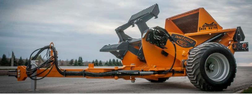
The SHoule Rock Gator rock picker offers many advantages versus the competition, including the ability to dump while in motion, the large bucket capacity and an unparalleled visibility while working.
