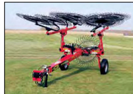
Rake in transport position with optional Center Kicker Wheel. 2200 series rake shown.
