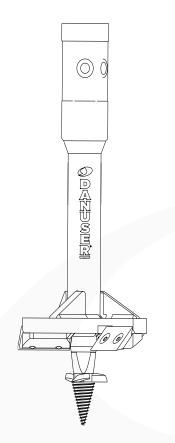
The stump auger planes away stumps without requiring large, specialized equipment. A threaded pilot digs into the stump and large cutting blades then shave the stump away. The large cutting blades are reversible for more cutting life. Complete stump removal is achieved by overlapping planning locations.
